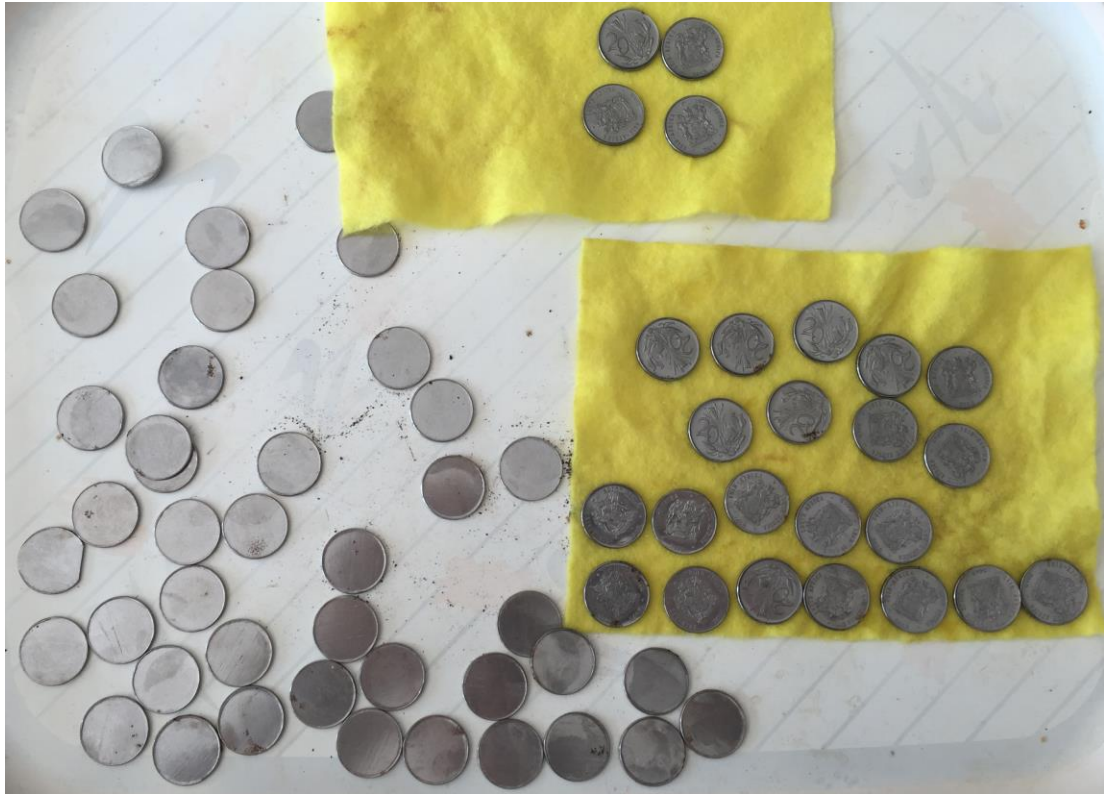
Figure 6. Planchets and 246B 20c patterns from the hoard examined by the author. The minted patterns are on the yellow cloth and the rest are planchets. Four of the patterns from this hoard are not shown in this photograph.
